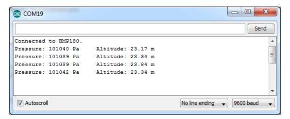
What you may have thought from the top description about pressure, is that it changes with temperature. This means in order to calculate our pressure correctly we need to know the temperature at which the measurement was taken. Luckily the BMP180 barometric pressure sensor has a temperature sensor inside. Inside our Love Electronics Arduino Library for the BMP180 Breakout Board we retrive the temperature when you ask for the pressure, so you
