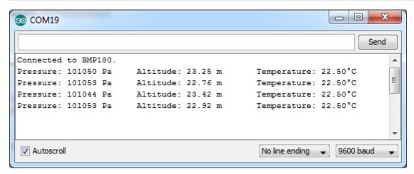
Great! Now we are collecting and outputting all the information the BMP180 sensor can collect, using only a few lines of code thanks to the Love Electronics BMP180 Arduino Library.
