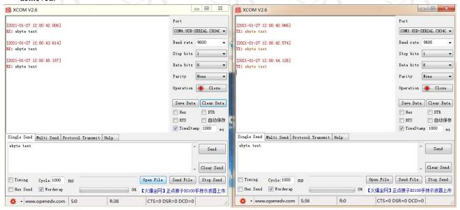
4、 User needs to open the mode switch first before link DTU with computer if the user want to modify parameters. Firing up <u>E32-DTU</u> 数传电台配置软件(E32-DTU parameter configuration application) to modify related parameters. The mode switch must be reopened to achieve transmission after the configuration.
